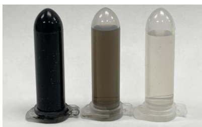
Commercial refillable black printer ink undiluted (left), diluted 1 : 10,000 (middle), and diluted 1 : 1,000,000 (right)
